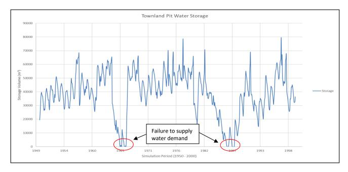
Figure 4-1 Townlands Open Pit storage between 1950 and 2000, assuming water is abstracted at 200 m³/day
